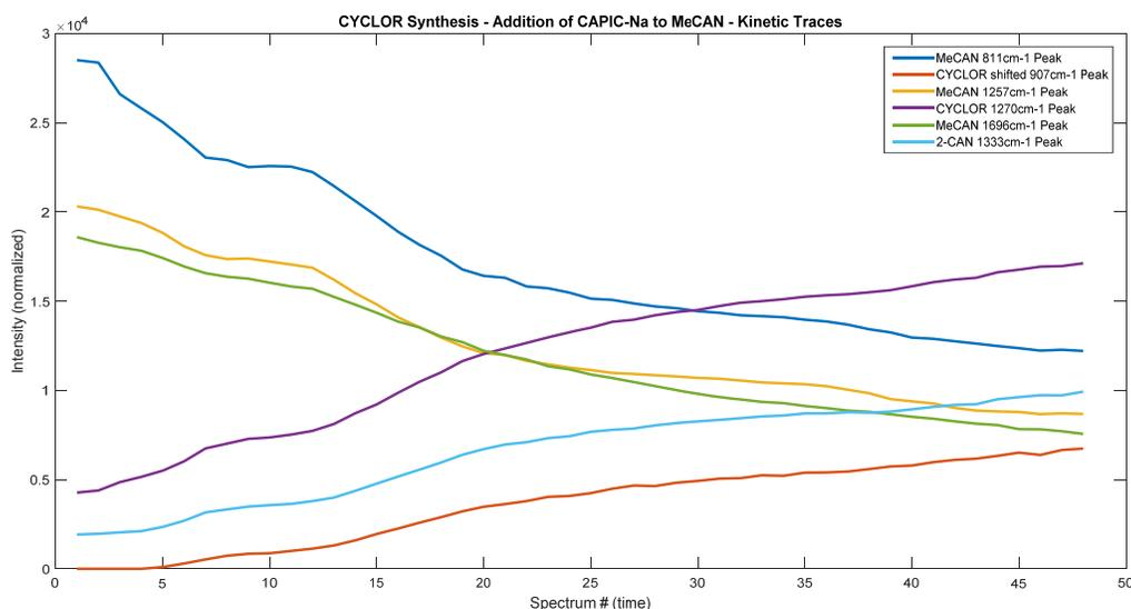
Figure 12: Selected peak traces revealing reaction kinetics
