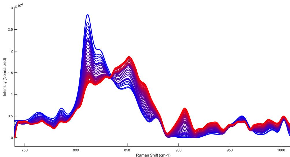
Figure 8: (Blue to Red  $\rightarrow$  time=0 to time=final) 750-1000 $\text{cm}^{-1}$  region
