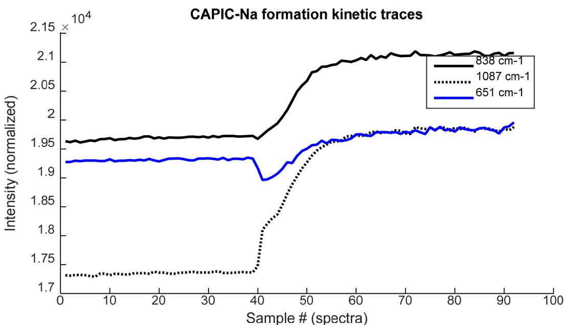
Figure 4: Kinetics traces of Raman peaks corresponding with formation of CAPIC-Na from CAPIC and NaH in diglyme
