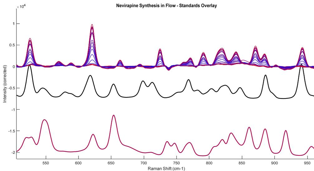
Figure 13: (Blue to Red → time=0 to time=final) Nevirapine flow synthesis, 500-950 $\text{cm}^{-1}$  region.
