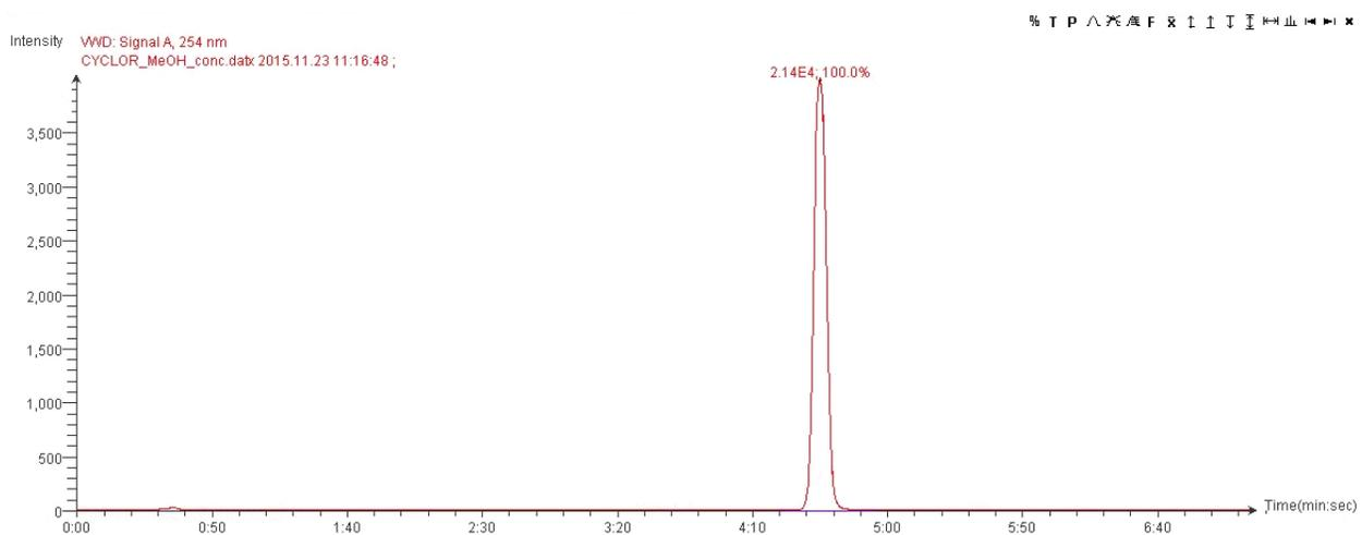
Figure 17: Chromatogram of pure CYCLOR in methanol, RT ~ 4:30 (mins:s)
