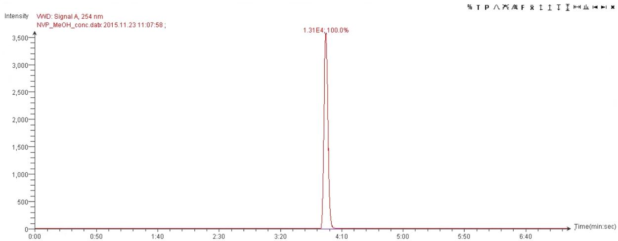
Figure 16: Chromatogram of pure nevirapine in methanol, RT ~ 3:55 (mins:s)
