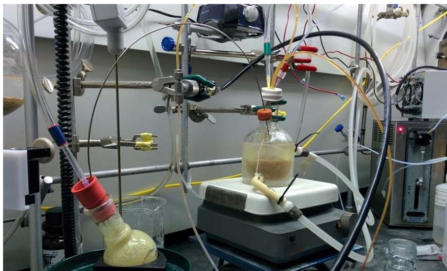
Figure 6: Experimental apparatus for synthesis of CYCLOR and online reaction monitoring with Raman Flow Cell (arrows indicate direction of flow of CAPIC-Na slurry and reaction mixture)
