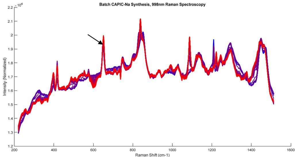
Figure 2: (Blue to Red → time=0 to time=final) Evolution of Raman spectra during batch CAPIC-Na synthesis
