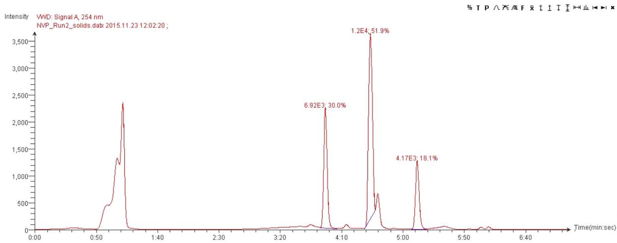
Figure 18: Chromatogram of crude output of packed NaH bed from nevirapine synthesis in flow
