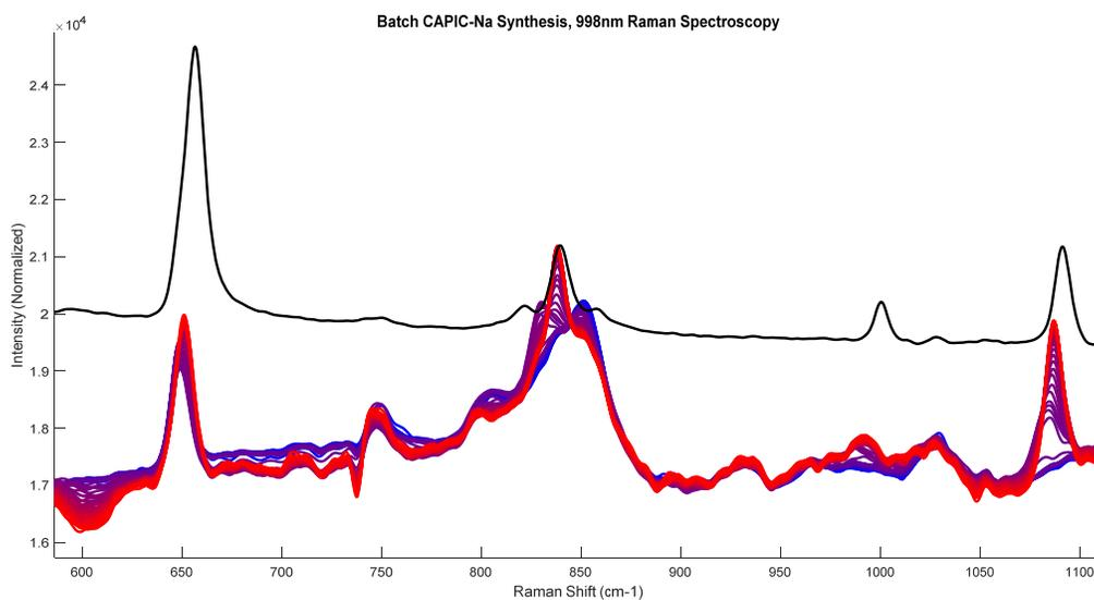
Figure 3: (Blue to Red → time=0 to time=final: black – pure CAPIC) Overlay of CAPIC spectrum with Batch CAPIC-Na spectra
