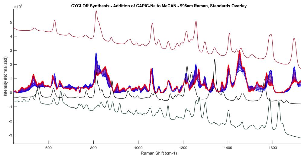
Figure 7: (Blue to Red → time=0 to time=final) Spectra acquired from Raman Flow Cell during addition of CAPIC-Na to MeCAN. Brown curve – MeCAN, black curve – 2-CAN, dark green curve – CYCLOR
