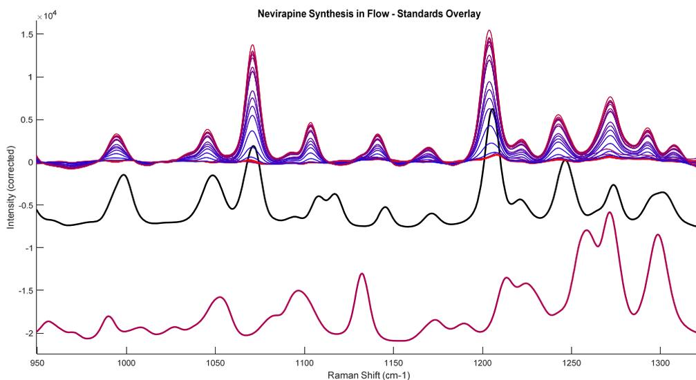
Figure 14: (Blue to Red → time=0 to time=final) Nevirapine flow synthesis, 950-1350 $\text{cm}^{-1}$  region.
